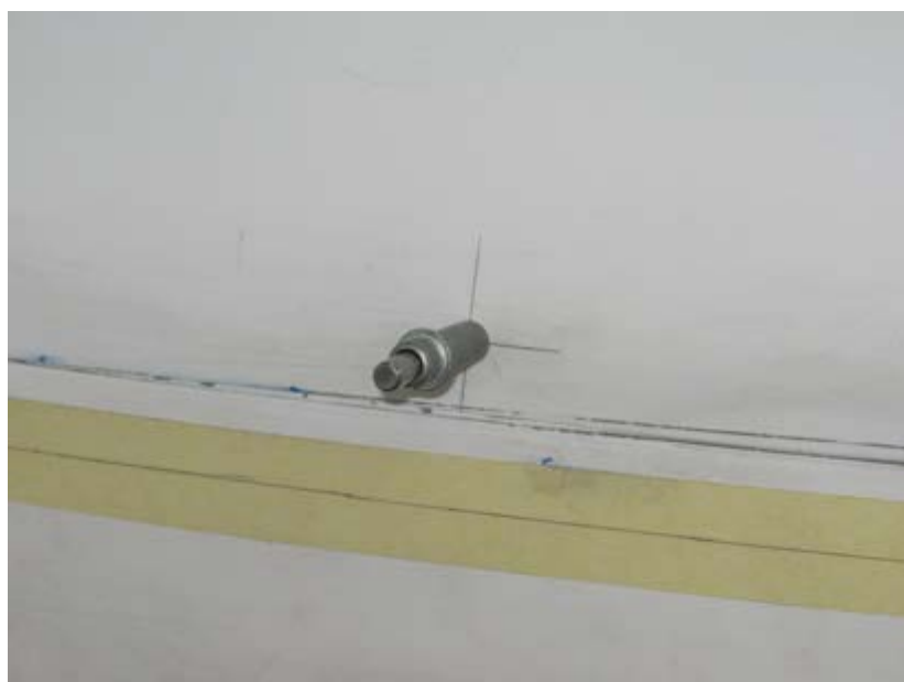
Figure 16: Fixing the lower and upper cowlings with cleco fasteners
