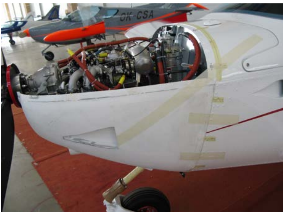
Figure 10: Fixing the lower cowling to the fuselage by masking tape
