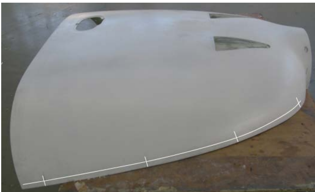
Figure 15: Hole midpoint marks for CAMLOC stud assemblies on the upper cowling
