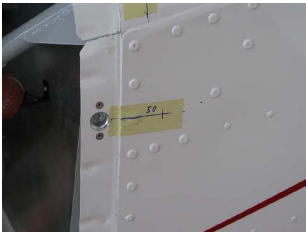
Figure 11: Helping line for hole midpoints – detail
