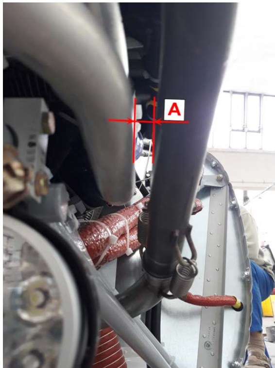
Figure 2: Distance between exhaust and thermostat valve
